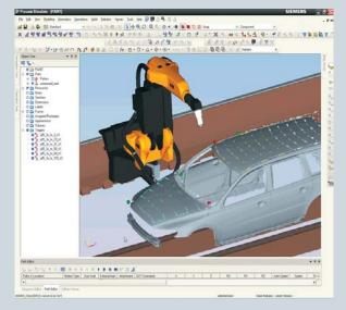
Process Simulate facilitates the design and validation of manufacturing processes in a 3D dynamic environment. Process Simulate is fully integrated
